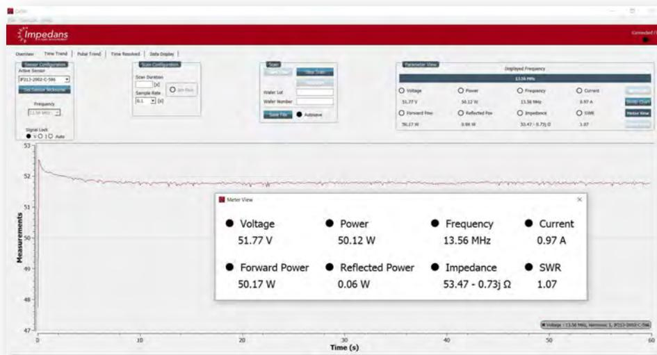
Figure 7: Example of the meter view.
